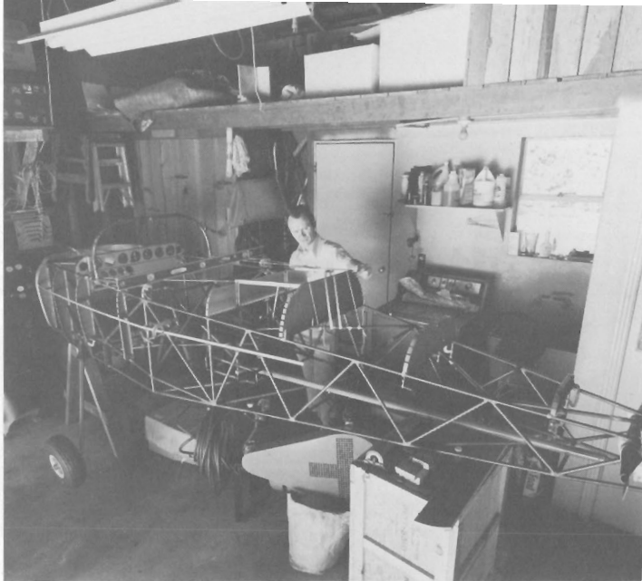
Jim Haynes of HP Labs, ready to install canopy slide rails on his Sidewinder, checks for alignment by using a piece of string. Jim, like most builders, doesn't have a big investment in equipment, but he has bought and refurbished some second-hand machine tools. By equipping his 125-horsepower engine with a constant-speed propeller, Jim expects a cruise speed of 170 miles per hour.
